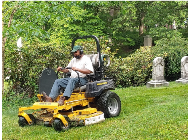
Figure 2. Gas mower that has been converted to propane. Note the tank behind the driver.
