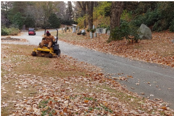
Figure 8 - Gas and propane powered mowers are adapted with special serrated blades to mulch the leaves in place. This adaptation has reduced the number of manhours required for fall clean-up each year and has also significantly improved the levels of organic matter and nutrients in the soil throughout the grounds.
