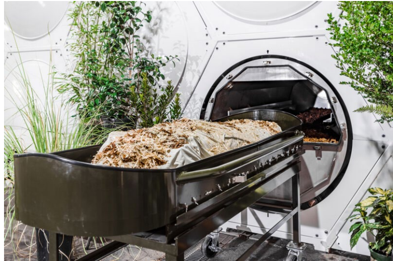
Figure 4 - Wood chips, alfalfa and straw cover a body which is then aerated to create an environment for microbes and essential bacteria. A body is reduced to compost within 30 days. Accessed March 8, 2021: https://religionnews.com/2021/02/10/recompose-nat
